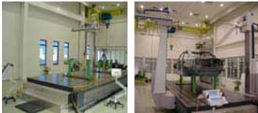
Latest measurement machine for body in whites
